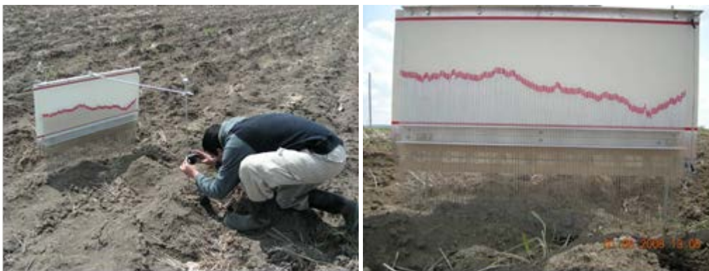
Figure 14. Capturing surface roughness with the roughness profilometer.
