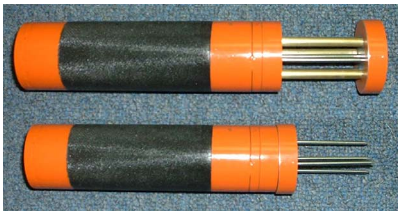
Figure 44: SMITY, Soil Moisture Insertion Tool, with slider extended and retracted.
