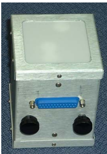
Figure 56. CROPSCAN Multispectral Radiometer (MSR). (Size is 8 X 8 X 10 cm).
