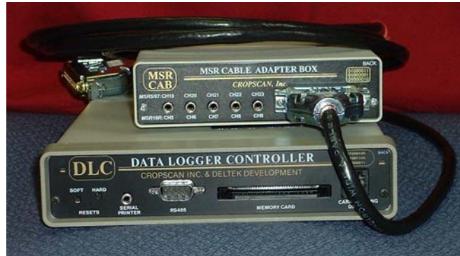
Figure 57. Data logger controller and cable adapter box.
