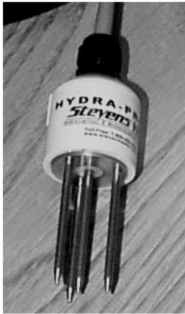
Figure 50. The Hydra probe used at the tower locations.
