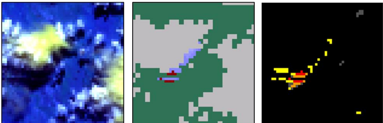
Figure 5. Example of snow commission associated with cloud periphery and shadowed surfaces. The left image (50 x 50 pixels) is a false color of VIIRS bands I1, I2, I3 subimage from NPP_VIAES_L1.A2017105.2012.001*.nc. The center image is the corresponding NDSI_Snow_Cover from VNP10.A2017105.2012.001*.nc (Fig. 1). Algorithm_bit_flags_QA set on to prevent snow commission error are shown as colored pixels in the right image.
